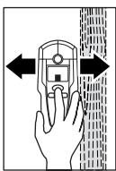
With the "**ZOOM**" button **4** pressed, move the measuring tool uniformly above the structure without lifting it off or changing the applied pressure. During the scan, the felt pads **8** must always have contact with the structure.
